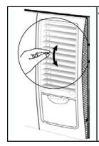
Airflow direction adjustment Up-and-Down.
